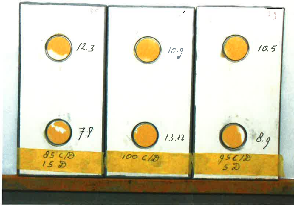
Photo 3: Panels after 720 hours Water Condensation test
