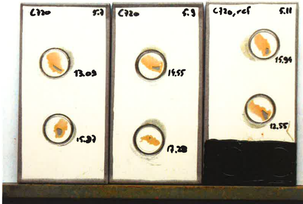
Photo 3: Panels after 720 hours Water Condensation test
