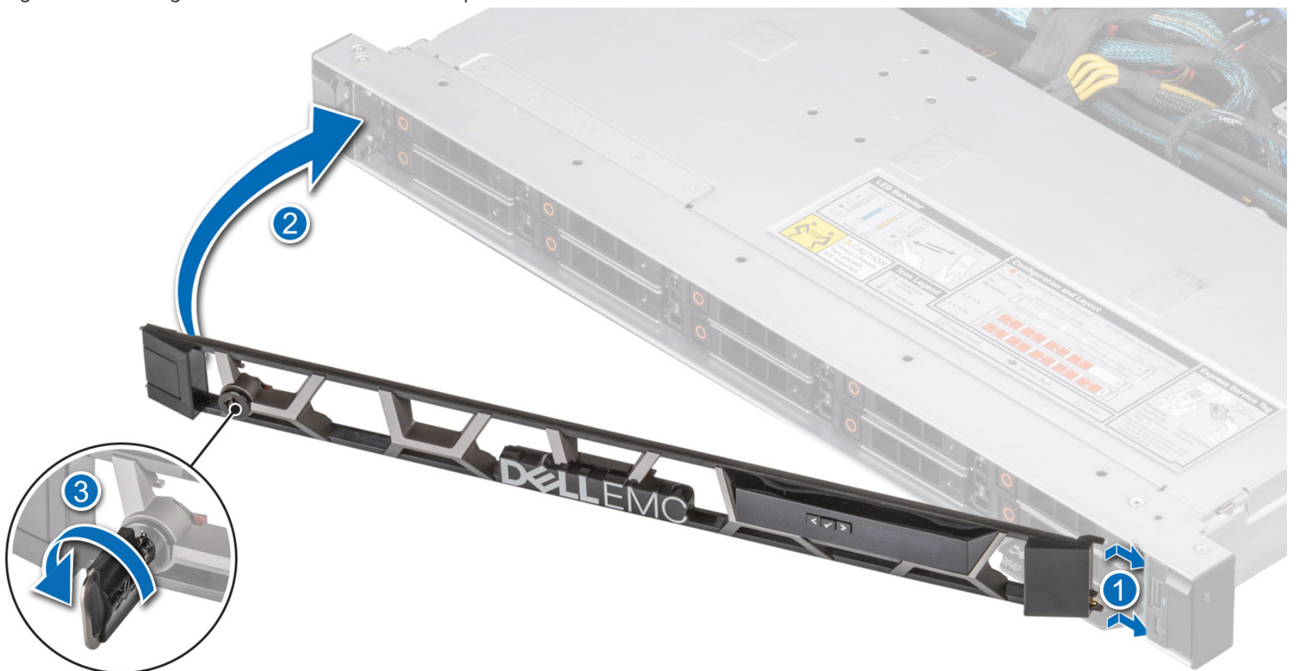
Figure 1. Installing the front bezel with the LCD panel
