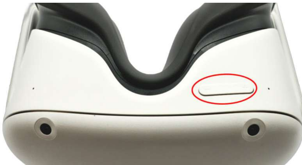
Fig. 5b. Volume buttons on underside of visor
