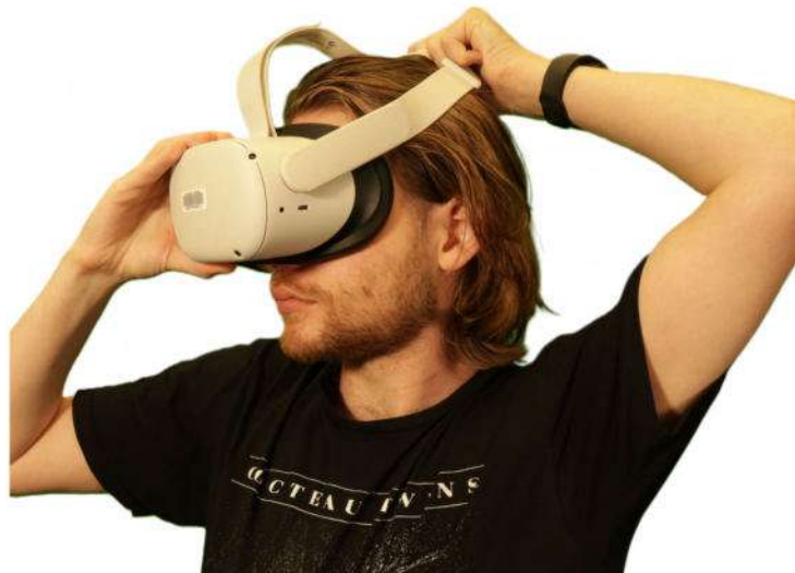
Fig. 1b. Headband being lowered/lifted
