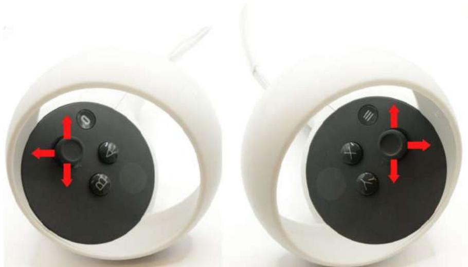
Fig. 4a. Controller analog sticks have 360-degree rotation
