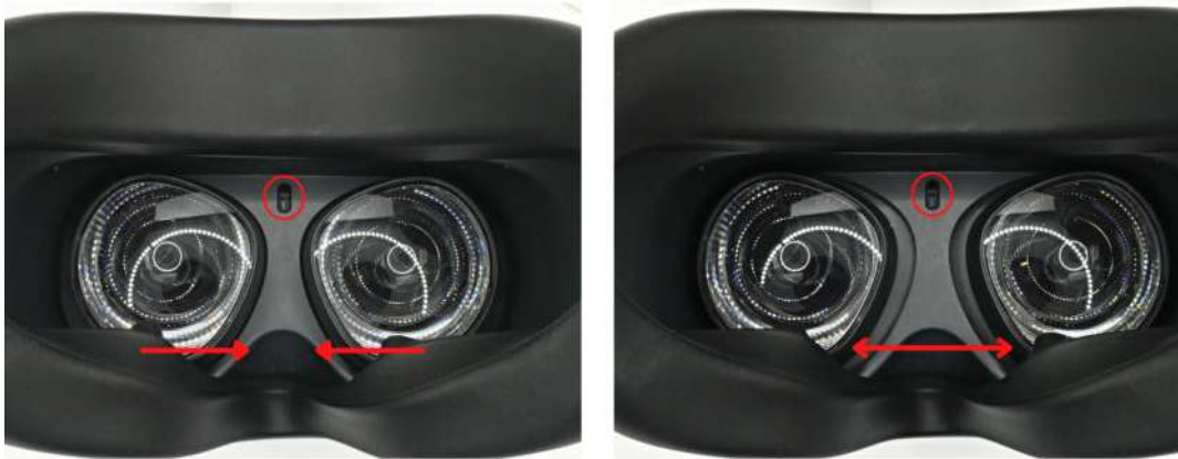
Fig. 5a. Lens-spacing slider inside visor
